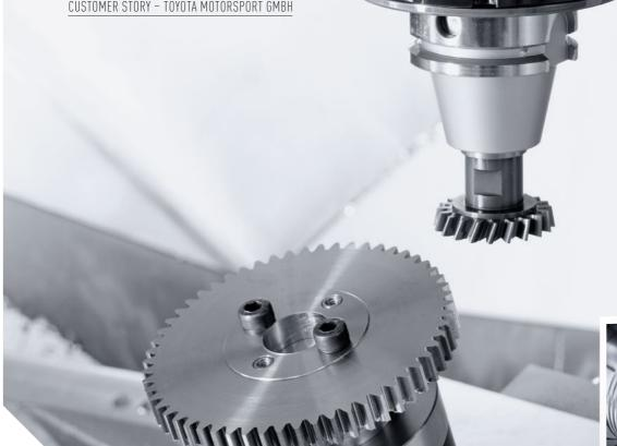
DMG MORI gearSKIVING - Machining of gears on a DMU 60 eVo to grinding quality.
