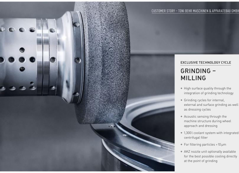
DMC 125 FD duoBLOCK including grinding package combines milling, turning and grinding in a single set-up.
