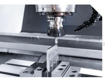
DINSE purchased two CMX 600 V centers for efficient 3-axis machining of prototypes and series parts.
