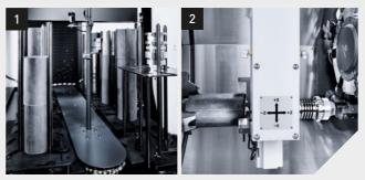
Stacking magazine 75 kg load capacity per pallet
