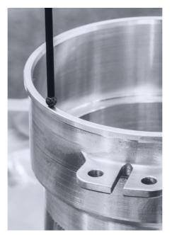
The highly safety-critical connectors undergo a 100 percent check for accuracy and cracks.
