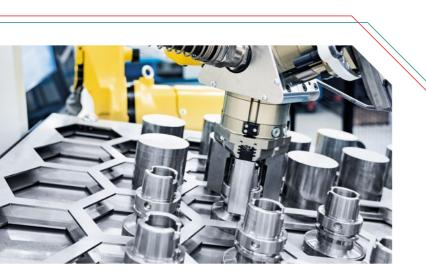
For different diameters, the Robo2Go automatically calculates the midpoint of the workpieces in order to grip them precisely.
