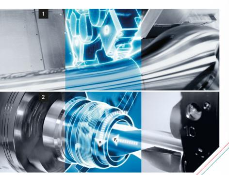
Selected DMG MORI technology cycles 1. Alternating speed: Avoidance of vibrations through specific variation of speed 2. Easy tool monitoring: Damage prevention in the case of tool breakage or overload
