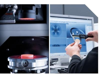
The LASERTEC 50 Shape undertakes applications that in many cases were previously only possible by spark erosion.
