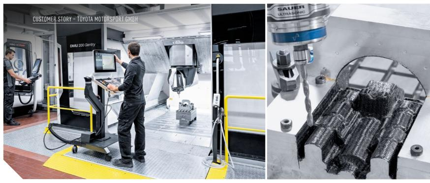
Installation of the DMU 200 Gantry in a pit to enable ground level loading and unloading of the delicate carbon fiber components with a forklift.
