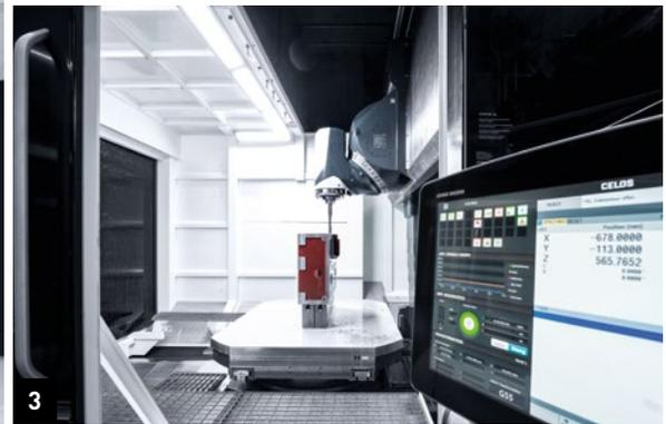
**1+2.** The volumetric accuracy of the DMU 210 U  $\mu$ Precision is 13  $\mu$ m and positioning accuracy is 4  $\mu$ m in all axes. **3.** A five-station pallet pool boosts the productivity of the DMU 210 U  $\mu$ Precision.
