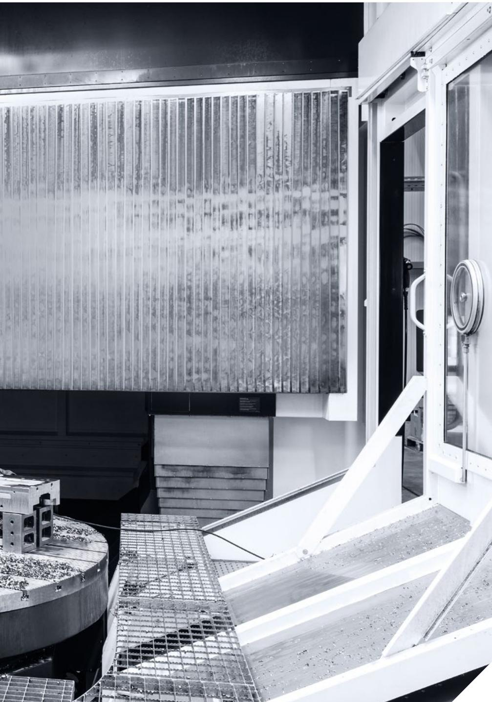
The work area of the DMU 340 P measures 3,400 x 3,400 x 1,600 mm. Maximum table load is 16 t.
